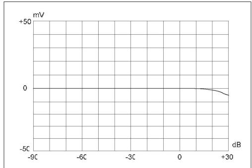
Figure 5. DC offset vs. gain, after symmetry adjustment
