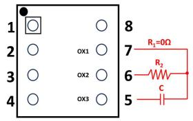
The MN3101 datasheet specifies an additional resistor ( $R_1$ ) on pin 7 to reduce power dissipation at higher frequencies. That additional resistor is not necessary for the CT3101 but it does not affect proper operation if present.
